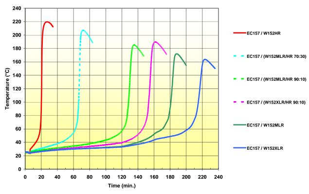
With HR label is identified the high reactivity hardener W152HR, generally utilized for small dimensions repairing or as reactivity modifier for the other W152 hardener.
