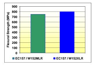
The laminate has been obtained by infusion of a  $600g/m^2$  glass E tissue. The specimens were obtained from the 5 mm thickness composites impregnated with the different system according to ASTM D790 and ASTM D2344 rules. Specimens were stabilized at  $50^{\circ}$ C for 16 hours before the test.
